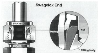
**Cross-Section of Swagelok End connection**
