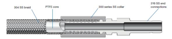
Swaged assembly method – There are two ways the hose end connections are supplied: Threaded end connection insert or non-threaded end connection insert:
